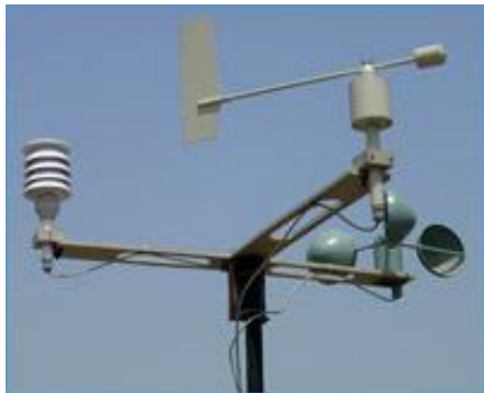
Wind monitor (wind speed, wind direction, T)
